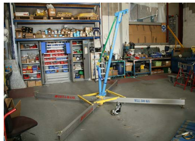
Figure 16 DAVIT INSERTED INTO SOCKET
