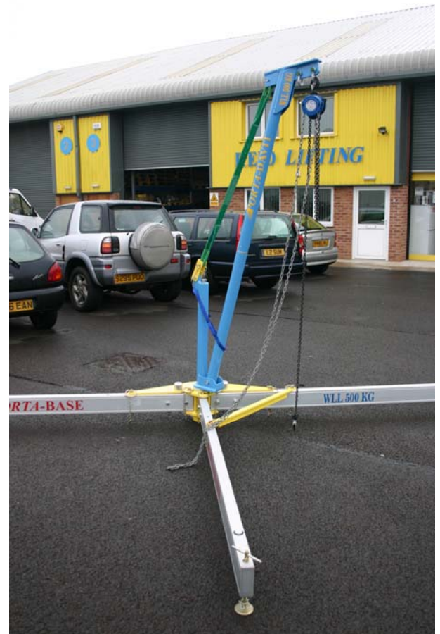
Figure 11 DAVIT INSERTED INTO SOCKET
