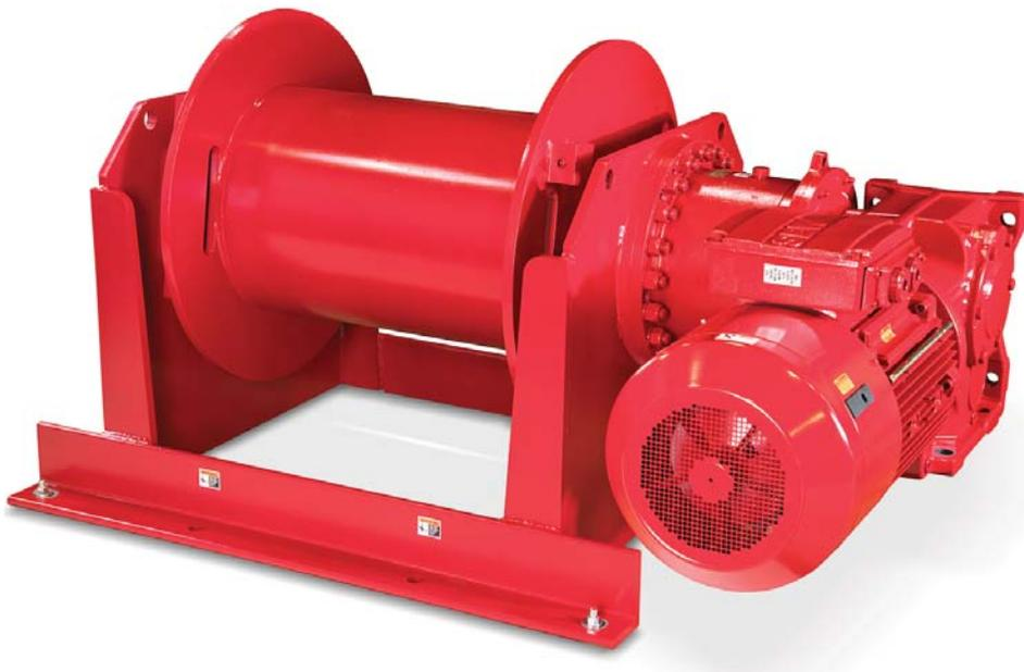
**WELDED STEEL DRUM** with flange anchors allow for uniform winding and help extend life of wire rope. Anchors allow cable to be over wound or under wound from either side of the drum.
