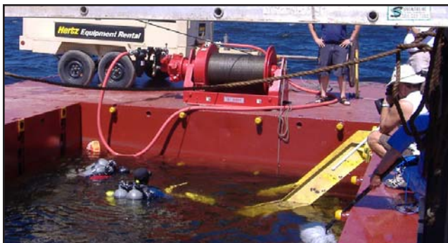
One of the two BIG RED air winches used on D&J's lift barge.
