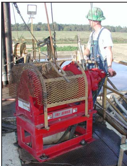
A worker operates a new TA series air winch.
